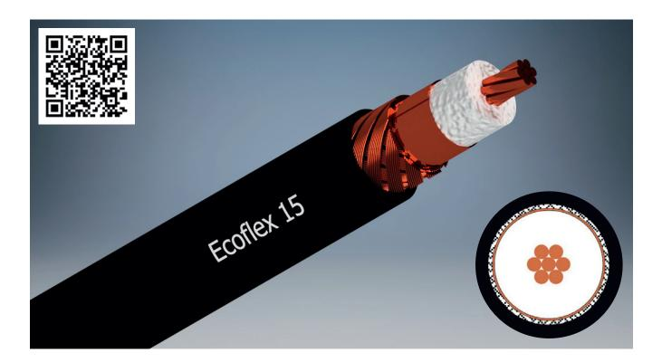
Ecoflex 15 is a flexible low loss 50 ohm coaxial cable for the frequency range up to 6 GHz. Advanced manufacturing techniques combined with the use of a low loss PE-LLC dielectric with a foaming rate of more than 70% result in very low attenuation values.
