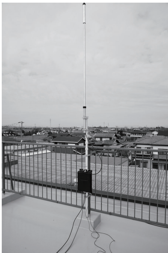
(Picture-1) Fixing the antenna mast (DAP600) at the support column of the hand rail, installing the element at the tip of the mast, fixing the ATU at the mast.
