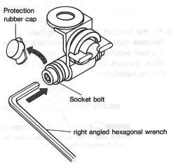
2. After loosening the bolt, hit the top of the wrench lightly. Hitting the wrench lightly will unlock the bolt and make it free to change installtion angle. Then adjust the bracket to make it vertical to road surface. To push lock nut at the oposite end will lock the bolt again. And hitting the bolt at the oposite end with the wrench will unlock the bolt.
