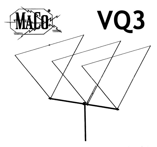
Maco introduces the new VQ3 V-Quad® Antenna that has been designed and tested by the Maco Engineering Department over the last 18 months. The VQ3 is a 3 element full wave antenna that is great for DXing. It is directional and can be used on horizontal and vertical polarization with one feed line. The VQ3 is tunable for 10 or 11 meters.
